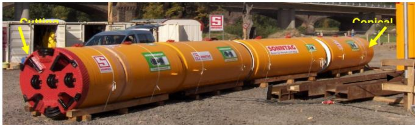
The Direct Pipe machine AVN1000XC for laying a 48"-pipeline
